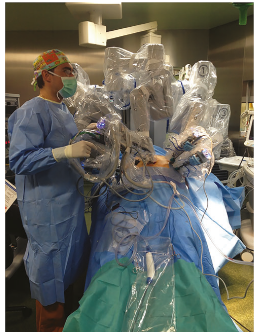
FIG. 2. da Vinci S™ system setup after docking during an RYGB. Please note the entrance of the motor-driven patient cart at the patient's head. RYGB, Roux-en-Y gastric bypass. Color images are available online.
