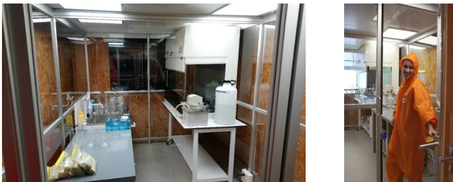
Fig. S3. 1. Clean laboratory for microplastic analysis at Institute of Environmental Sciences and Technology- Autonomous University of Barcelona, and example of the coverall wore during sample preparation.
