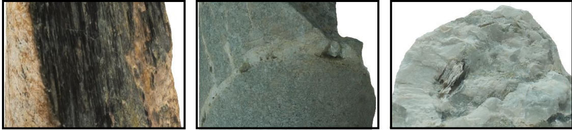
Figure 49. Examples of zoomed screenshots of the textured 3D model of three different borehole samples.
