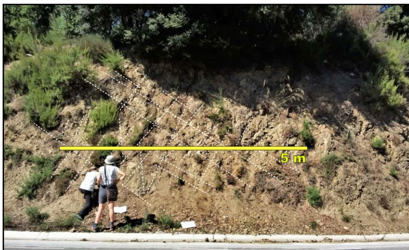
Figure 41. Example of fracture/discontinuity identification in a granodioritic outcrop, using the scanline method. Dashed white lines highlight main fractures.
