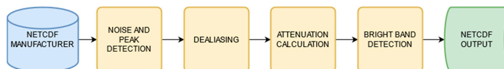
Figure 2. Flowchart of the new processing methodology.
