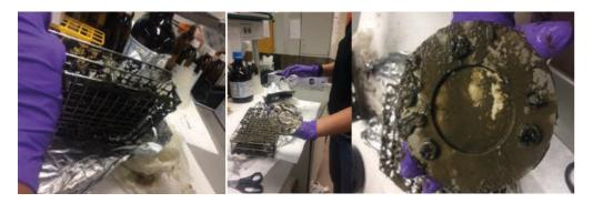
Figure S2: Appearance of the POCIS once transported to the laboratory and dismantled for subsequent cleaning and extraction.
