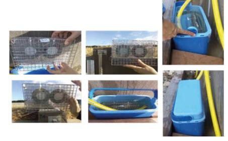
Figure S1: Installation of the POCIS at the outlet of the SAT system T4.
