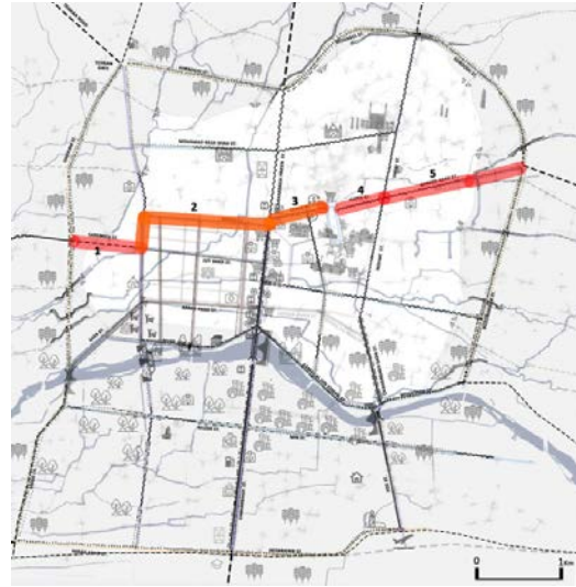
Fig. 186. The extension of the main horizontal axis. (1) Khiaban-e-Saremieh, (2) Khiaban-e-Khosh, (3) Khiaban-e-Sepah, (4) Khiaban-e-Hafez, (5) Khiaban-e-Ahmad Abad, (Red lines- Demolition and crossing over residential fabric), (Orange lines- Widening the existing ground passages)
