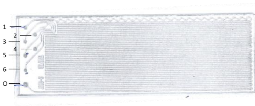
Figure 109: Active Droplet Manchip 2 Assay chip with respective inlets and outlet. The chip has an overall length of 2.28 m and a dual-channel spacing of 600 \mu\text{m}
