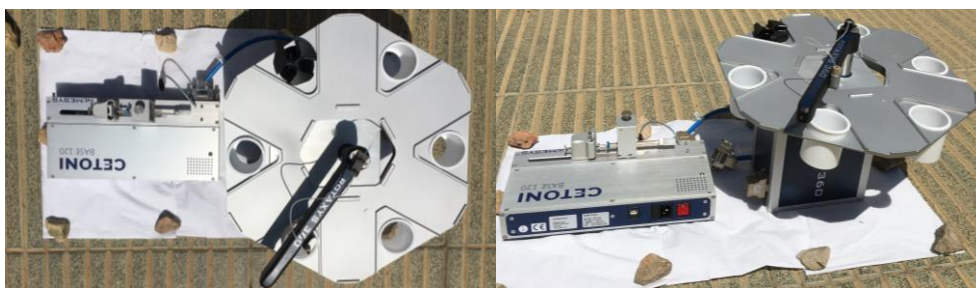
Figure 57: ROTAXYS 360 LHS equipped with a base module 120 and a neMESY low-pressure syringe opted for 100 \mu l max volume.
