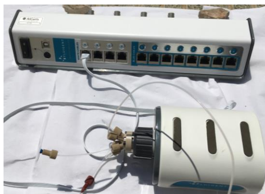
Figure 53: L-Switch™ switch with depicted interface. The 6 port/ bidirectional valve allowed the automated switch between independent flows.
