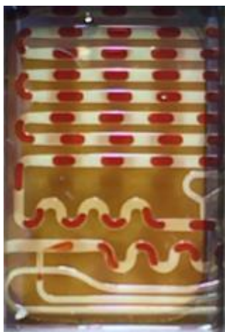
Figure 124: Mixing of 0.67 mM Fe(NO 3 ) and 2 mM KSCN in droplets in tetradecane with 0.5 % SPAN 20. Droplet generation was recorded with 200 frames per second using the mobile camera of an iPhone 5 SE.
