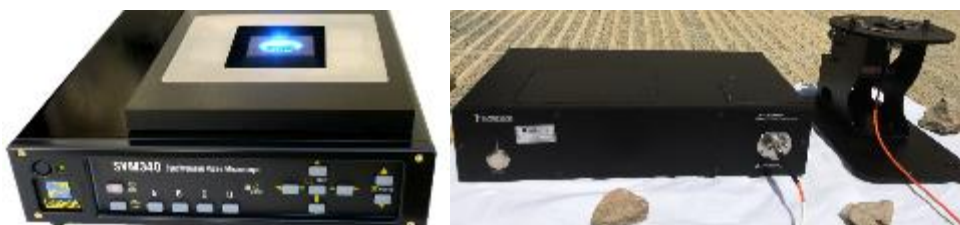
Figure 38: Optical readout devices provided by microfluidic companies. On the left: OptoReader from Elveflow connected to the 3D alignment platform with a duplex optical fiber cable. On the right, SCM340 from LabSmith.
