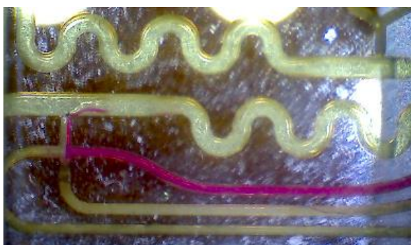
Figure 122: Droplet formation with tetradecane + 0.5 % Span 20 as the CP and a mixture of 0.5 % phenolphthalein in 20 mM HEPES (pH 9) and 0.1 M HCL as the DP in the VIM2 microreactor. Taylor dispersion leads to the fast mixing ( <150 ms) of the two water phases, leading to phenolphthalein's protonation and discoloration.
