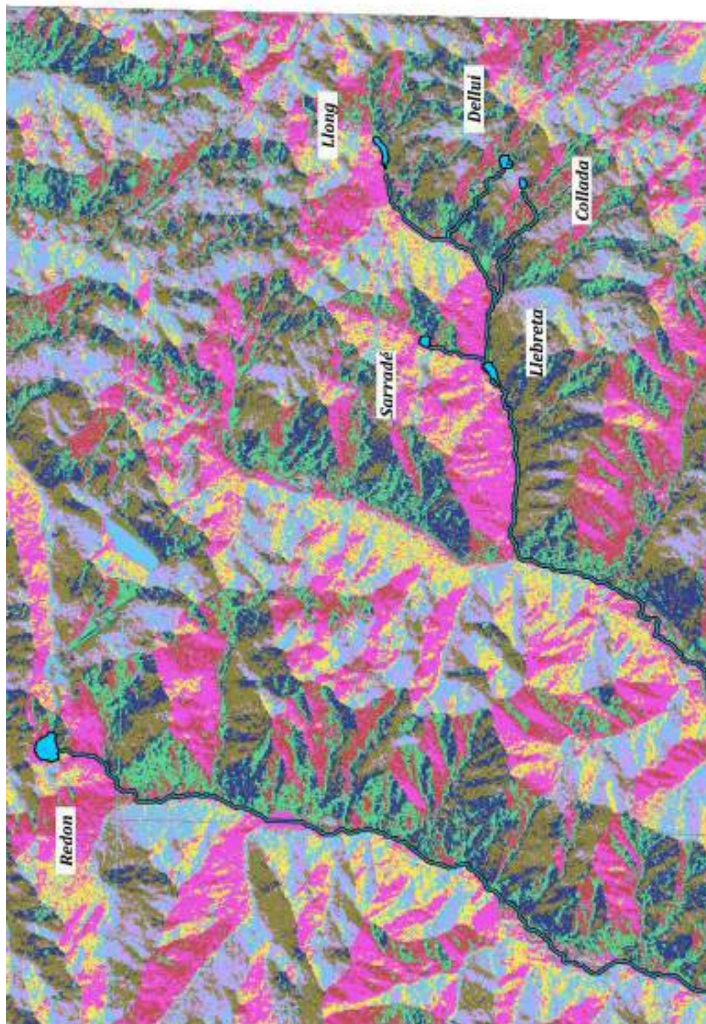
Figure 45. Flow direction grid for the calculation of water drainage pathways in the area of study. Each colour represents a different slope direction. The lakes and main drainage streams have been superimposed for reference. Calculations performed and figure created using the Arc Hydro data model and toolset in ArcGIS (Esri, Redlands, CA, USA). Calculations performed using ASTER GDEM data (ASTGTM v002, doi.org/10.5067/ASTER/ASTGTM.002 ). ASTER GDEM is a product of the Ministry of Economy, Trade, and Industry (METI) of Japan and the United States National Aeronautics and Space Administration (NASA).
