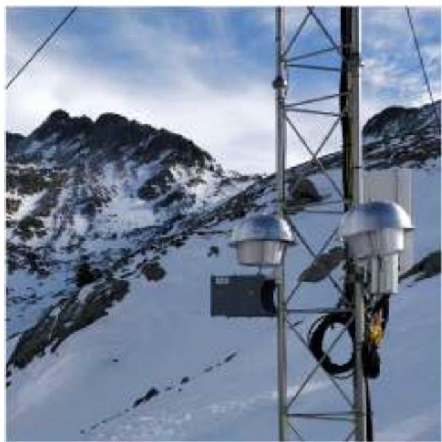
Fig. 1. PUF-PAS samplers deployed in the Pyrenees (2240 m.a.s.l.) inside dome-shaped stainless steel housings affixed to the structure of an automatic weather station.
