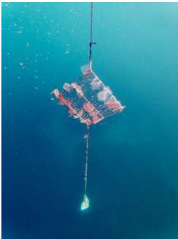
Fig. 2. Low-density polyethylene passive water samplers (LDPE-PWS) after a year of deployment below the water surface. The LDPE sheets were mounted onto a stainless-steel rack held four meters below the surface by a buoy and a heavy weight.
