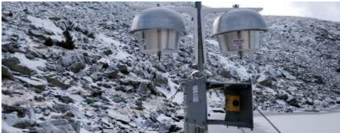
Figure 19. Data logger (Tinytag Plus 2, yellow box) deployed at each studied site for registering the ambient temperature and relative humidity for the duration of the sampling periods.
