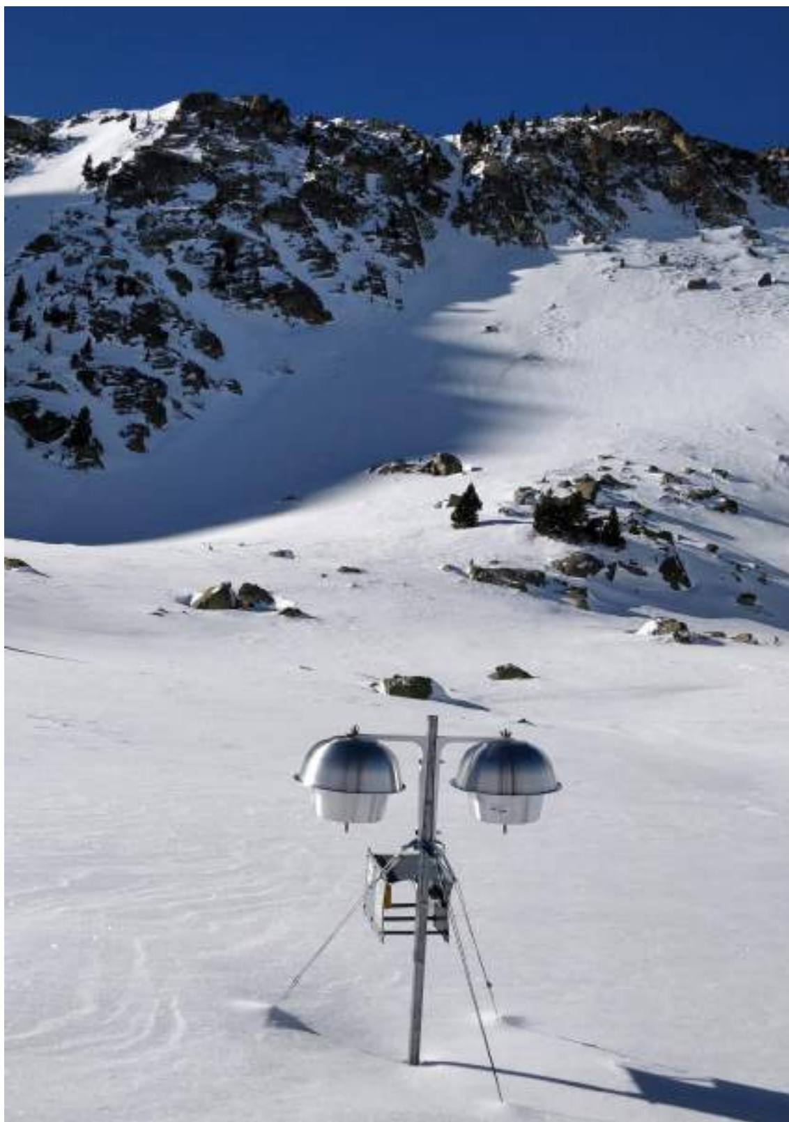
Figure 26. Passive air samplers deployed at Estany de la Collada.
