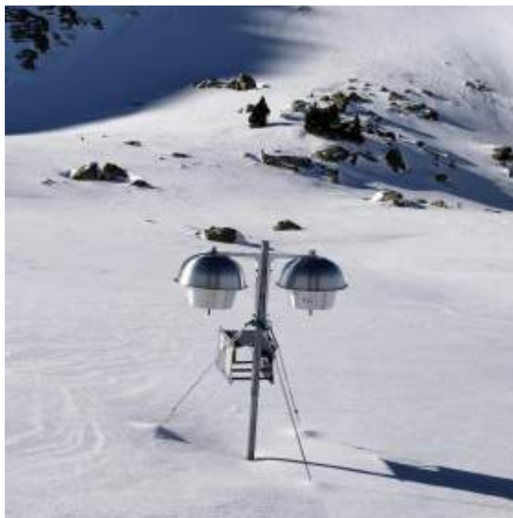
Figure S4.1. Polyurethane foam passive air samplers (PAS-PUFs) inside stainless steel dome housings near lake Collada (2,453 m asl) during January 2018.
