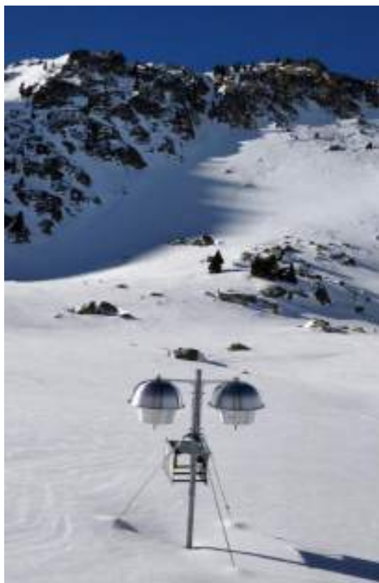
Figure S3.1. Polyurethane foam passive air samplers (PUF-PAS) were deployed in duplicate inside of steel dome housings held 1.8 m above ground. In the picture, samplers deployed during winter 2017-2018 near lake Collada in the Catalan Pyrenees (2,453 m.a.s.l.).
