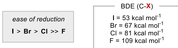
Figure 4.1.4. Bond dissociation energy is a factor that can predict ease of reduction.
