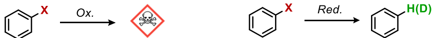
Figure 4.1.2. Oxidation leads to highly toxic compounds, whereas reduction can allow for incineration
