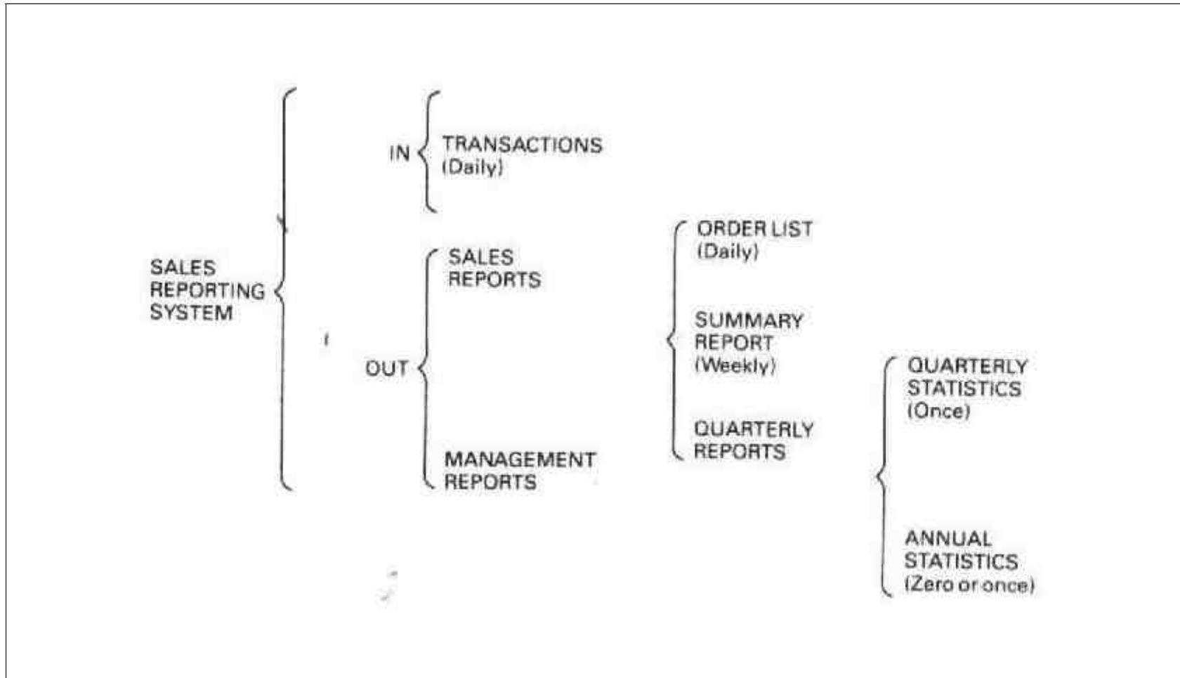
Diagrama Work breakdown structure
