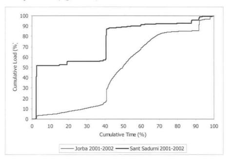
Figure 5-27: Cumulative time against cumulative load during 2002-2003 at both sampling sites
