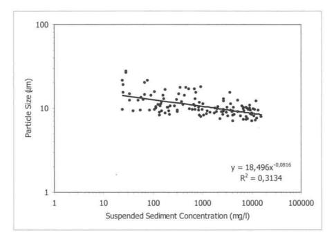
Figure 4.4-3: Particle size against suspended sediment concentration relationship.
