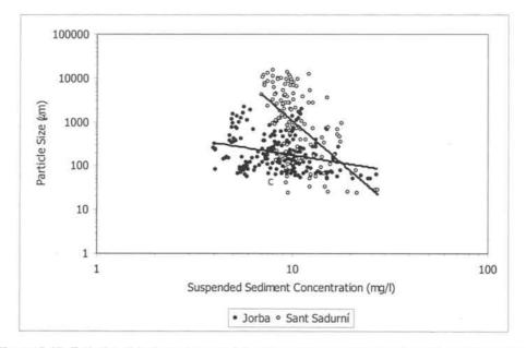
Figure 5-17: Relationship between particle size and suspended sediment concentration.
