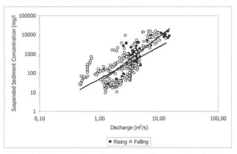
Figure 4.2-12: General rising and falling stage rating curve at Sant Sadurní.
