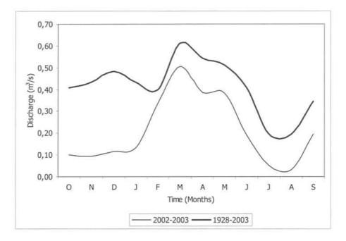
Figure 2-30: Discharge pattern at Jorba during 2002-2003 and the mean monthly discharge
