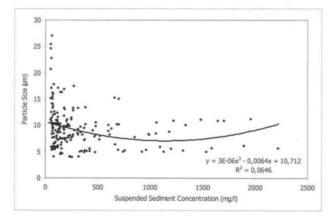
Figure 4.3-2: Particle size against suspended sediment concentration relationship
