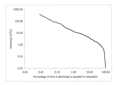
Figure 2-31: Frequency duration curve of discharge at Sant Sadurní.
