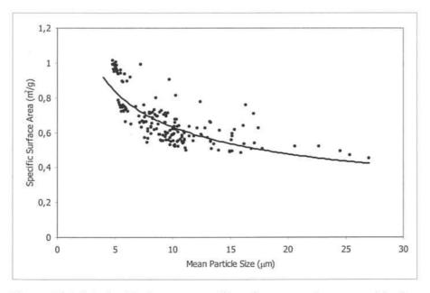
Figure 4.3-4: Relationship between specific surface area and mean particle size.
