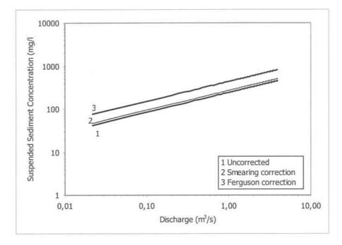
Figure 3-4: Uncorrected data, Smearing correction and Ferguson correction at Jorba.
