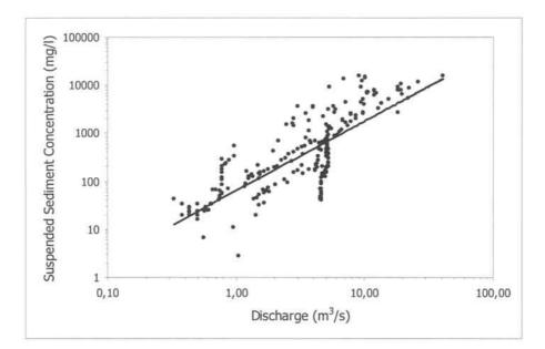
Figure 4.2-9: Suspended sediment rating curve at Sant Sadurní during 2002-2003
