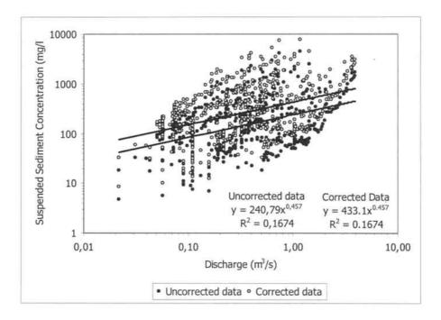
Figure 3-2: Uncorrected and corrected concentration data at Sant Sadurní
