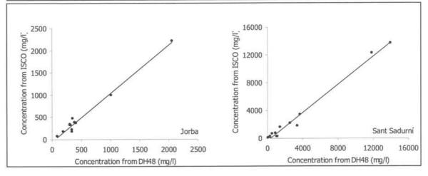
Figure 3-1: Calibration of the ISCO samples versus de manual samples at Jorba and Sant Sadurní.
