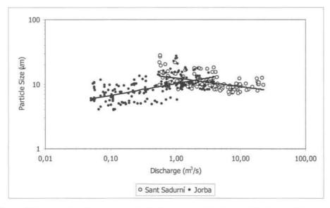
Figure 5-15: Relationship between particle size and discharge at both sampling sites.
