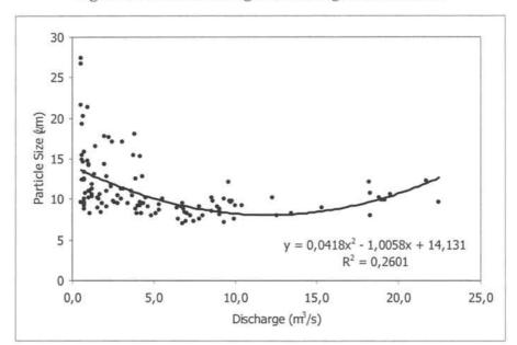
Figure 4.4-2: Polynomial adjustment of particle size and discharge relationship at Sant Sadurní
