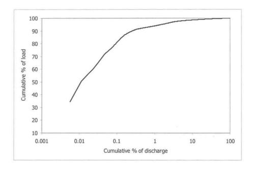
Figure 4.6-1: Cumulative % of load versus cumulative % of discharge
