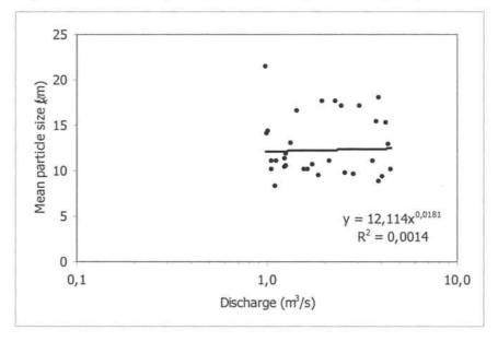
Figure 4.4-15: Relationship between particle size and discharge of the event.
