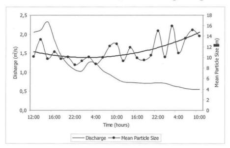
Figure 4.3-16: Evolution of mean particle size with discharge.
