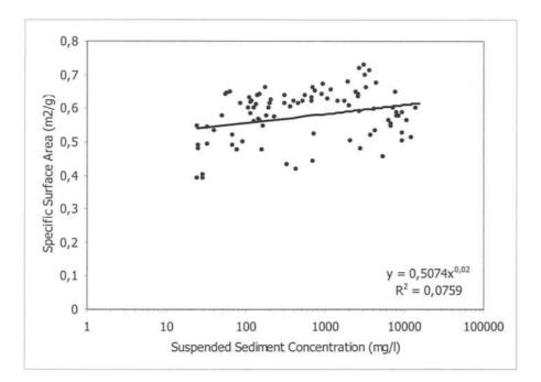
Figure 4.4-7: Specific Surface area and suspended sediment concentration relationship at Sant Sadurní during the study period
