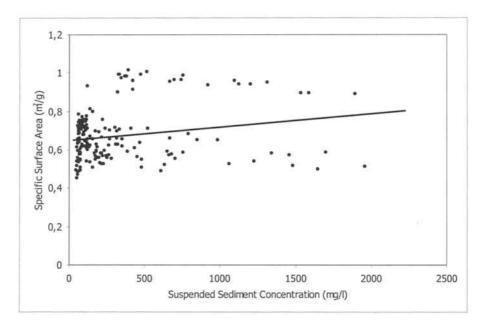
Figure 4.3-6: Relationship between specific surface area and suspended sediment concentration.
