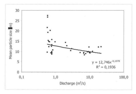
Figure 4.4-11: Relationship between discharge and particle size
