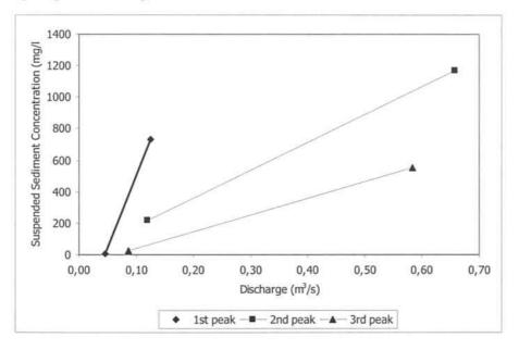
Figure 4.1-17: Slope between the maximum and minimum concentration in the successive peaks.
