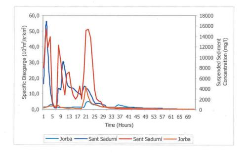
Figure 5-8: Evolution of specific discharge and sediment concentration at both sampling sites during the event.
