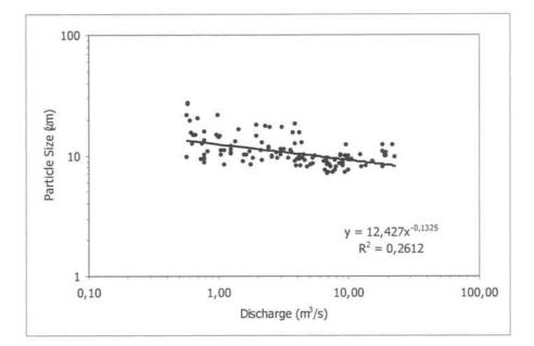
Figure 4.4-1: Particle size against discharge at Sant Sadurní
