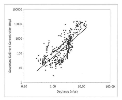
Figure 4.2-6: Suspended sediment Rating Curve at Sant Sadurní.
