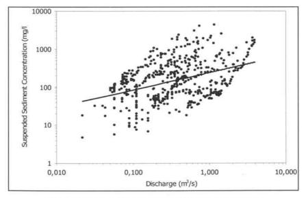
Figure 4.1-5: Suspended Sediment Rating Curve at Jorba
