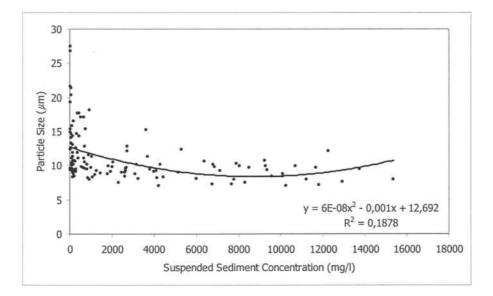
Figure 4.4-4: Particle size against suspended sediment concentration with a polynomial adjustment
