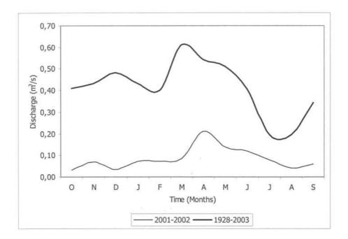
Figure 2-29: Discharge pattern at Jorba during 2001-2002 and the mean monthly discharge
