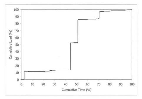
Figure 4.6-2: Cumulative % of time versus cumulative % of load
