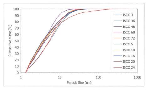
Figure 4.3-17: Particle size distribution for individual samples
