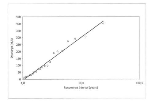
Figure 2-20: Recurrence interval of instantaneous peak discharge at Sant Sadurní.
