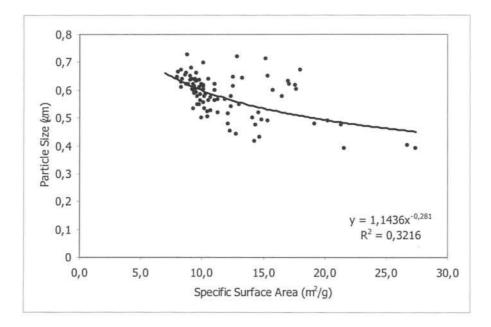
Figure 4.4-5: Relationship between Particle size and specific surface area at Sant Sadurní
