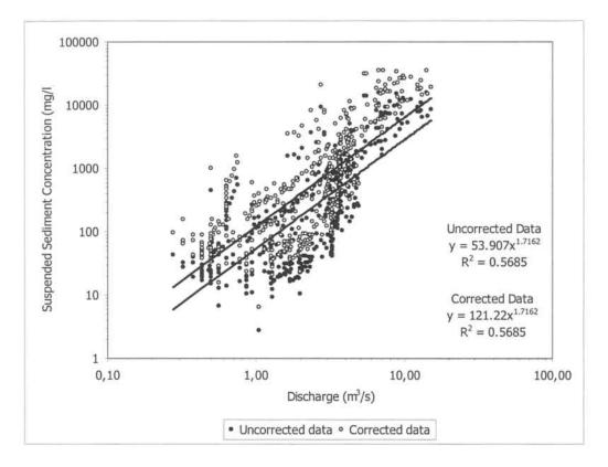
Figure 3-3: Uncorrected and corrected concentration data at Jorba.
