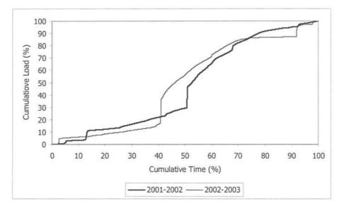
Figure 4.6-7: Cumulative load versus Cumulative Time for 2001-2002 and 2002-2003
