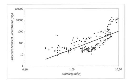
Figure 4.2-8: Suspended sediment rating curve at Sant Sadurní during 2001-2002
