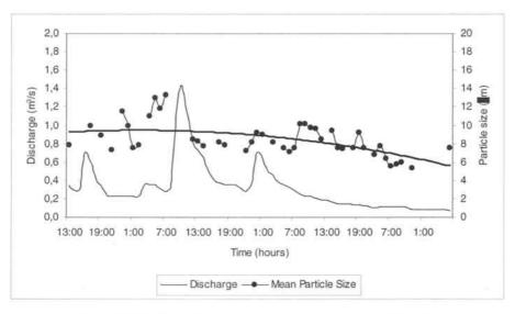
Figure 4.3-10: Evolution between discharge and particle size
