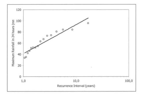
Figure 2-18: Recurrence Interval for the maximum rainfall in 24 hours at Sant Sadurní.
