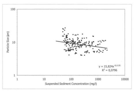
Figure 4.3-3: Particle size against suspended sediment concentration in a log-log chart.
