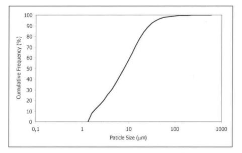
Figure 4.4-17: Mean particle size distribution at Sant Sadurní.
