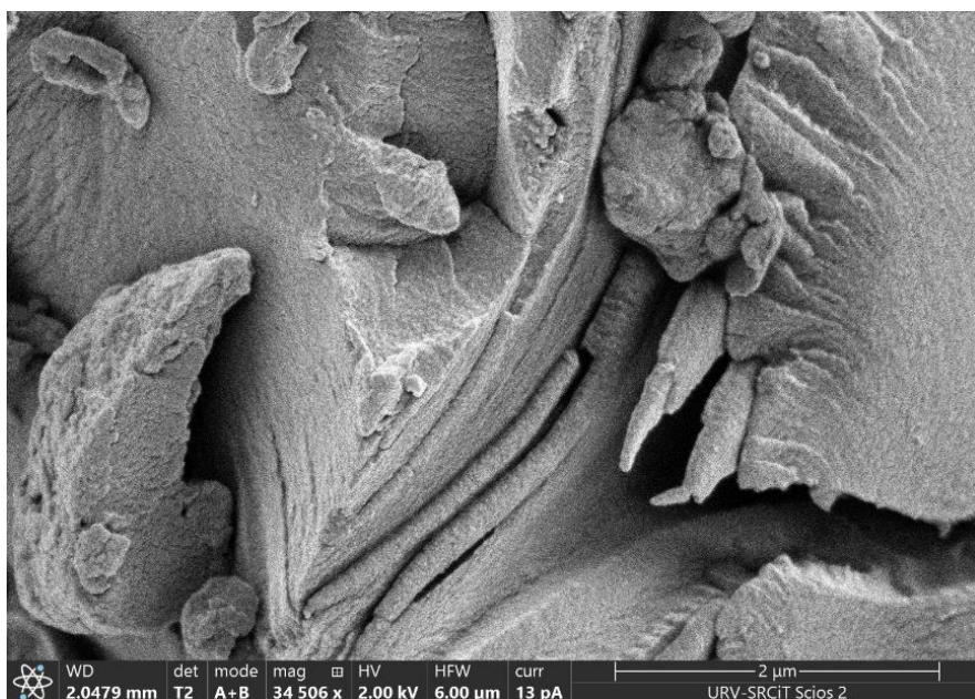
Annex 4.9 FESEM images of PMDA-β-CD-NS seen at a scale of 500 nm (top) and at lower magnification (bottom)
