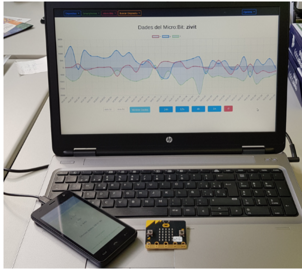
Figure 10.6: Prototype of the e-PEMICU platform, showing the motion data collected by a micro:bit sensor (reprinted from [159]).
