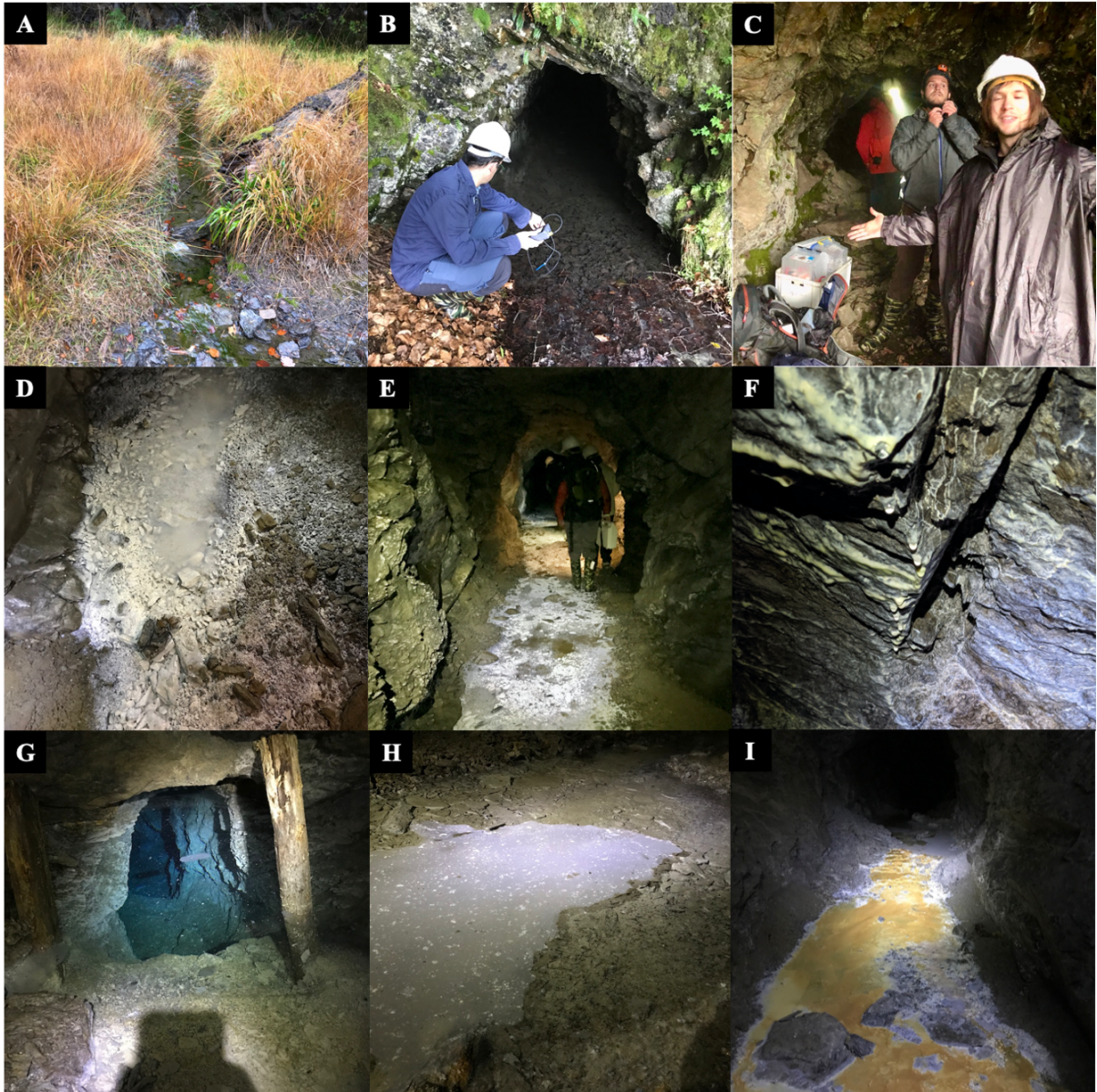
Figure 2.6. Photos taken from inside and outside of the Victoria Mine during the 2019 campaign. From A to I represents walking "upstream" with respect to the flow of water (i.e. moving deeper into the gallery). (A) Melics Creek nine meters downstream from where the mine effluent merges (sample-3). Microbial DNA was sampled here in 2019. (B) Jordi Cama measuring pH at the entrance of the Sinçay Gallery/mine effluent (sample-4). (C) The entrance of the 1330 Gallery. (D) 65 m from the gallery entrance and the first occurrence of flowing water and actively precipitating hydrozincite. Microbial DNA was sampled here in 2019. (E) \approx 100 meters from the gallery entrance. Water is flowing on the floor and hydrozincite is present. (F) Drip water at 140 m from the entrance (sample-6). (G) 160 m from the entrance where a shaft is flooded (sample-7). (H) \approx 170 m from the gallery entrance where the "floating skin" morphology of hydrozincite can be observed. The white mineralization is floating on top of the water. This is ubiquitous throughout the gallery. (I) 190 m from the entrance and the first occurrence of a reddish precipitate (sample-8).
