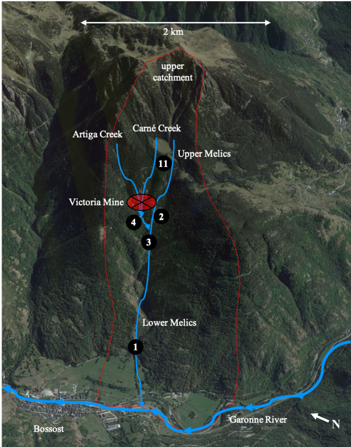
Figure 2.4. Google Earth image of the Victoria Mine catchment system and locations of outdoor sampling intervals. Sampling locations correspond to Table 2.1 and Figure 2.5, however sample locations 5-10 are omitted. The red line represents the catchment boundaries and the red oval with the "X" is the approximate location of the Victoria Mine. Artiga Creek was never sampled because it was dry during all three sampling campaigns. Blue arrows represent water and the corresponding flow direction.
