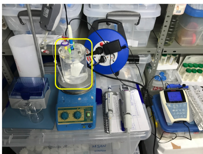
Figure 2.9. (left) A photo taken of the batch dissolution experiment at 3.7°C inside of a walk-in cooler. The white angular mineral suspended in the liquid is a sample of the floating skin hydrozincite (Figure 2.8(3)). (right) A schematic of the batch experiment showing the constant air bubbling and stirring, while the pH meter was fixed in position for in-situ measurements. The sample port was maintained closed while sampling was not occurring, and there was an outlet hole for air to escape so as not to build pressure within the vessel.
