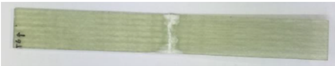
FIGURE 6.21: Failure of a specimen for the longitudinal flexural testing, damage localised in the centre.
