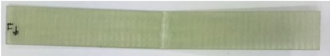
FIGURE 6.23: Failure of a specimen for the transverse flexural testing, damage localised in the centre.
