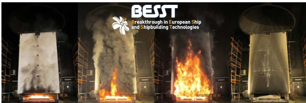
FIGURE 1.3: Experimental testing of a wall-fire extracted from the BESST project [2].
