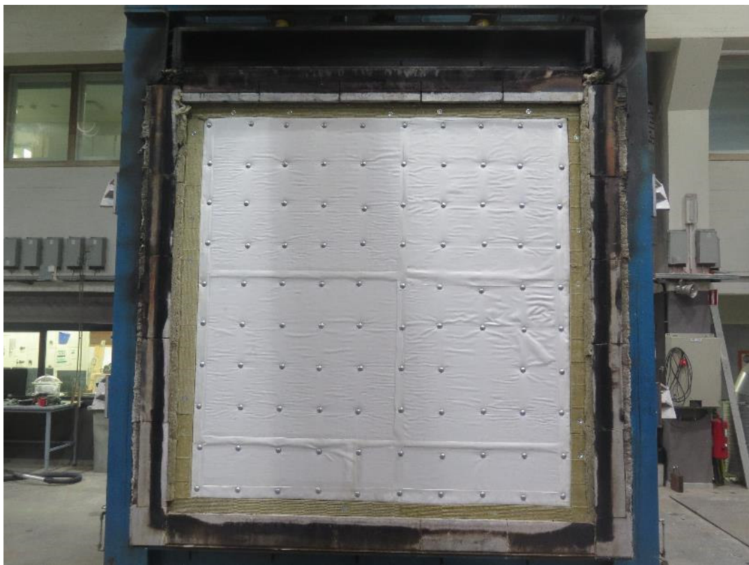
FIGURE 6.62: Experimental setup for the bulkhead test. Picture by courtesy of Eurofins Expert Services.
