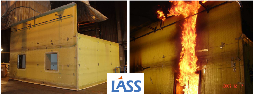
FIGURE 1.4: Experimental testing of a superstructure room extracted from the LASS project [3].
