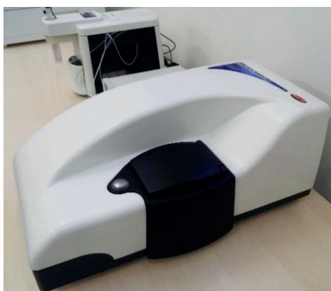
Figure 26: ZetaSizer Nano ZS equipment (Malvern Panalytical, Netherlands, and United Kingdom) for DLS analysis carried out in present studies.
