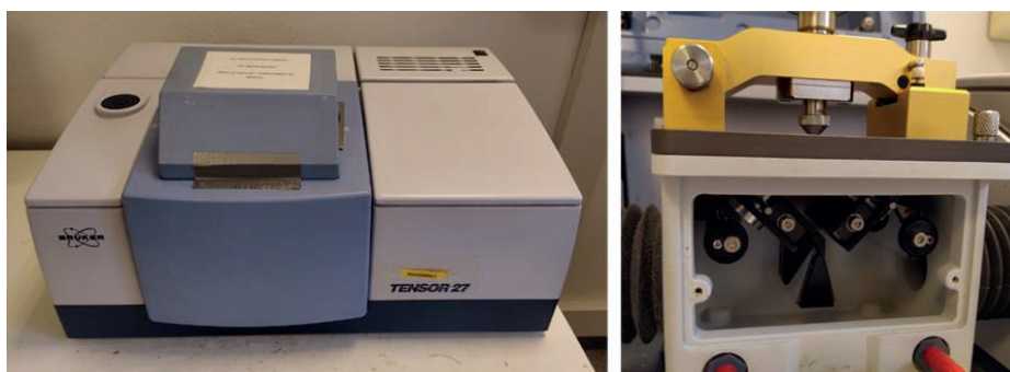
Figure 23: Infrared Spectrophotometer Tensor 27 (left) equipped with an Attenuated Total Reflectance module Specac Golden Gate (right) used in the present studies.
