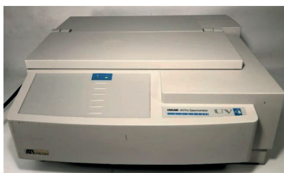
Figure 17: UNICAM UV-2 200, UV double-beam spectrophotometer used in present studies.
