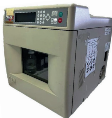
Figure 15: CEM corporation MARS 5 digestion analytical microwave system (CEM Corporation Matthews, North Carolina, USA) used in the present studies.
