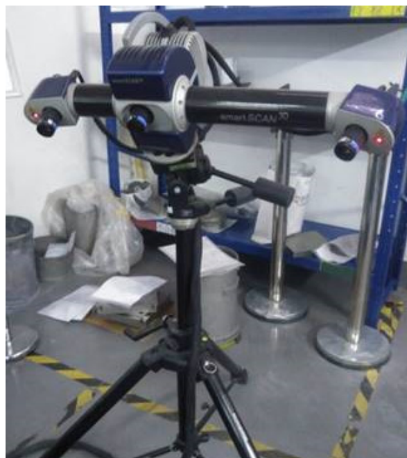
Figure 2. Breuckmann SmartSCAN3D scanner for the warpage measurements.
