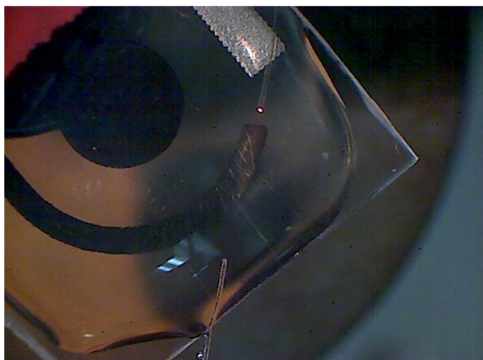
Figure 8.12: Image highlighting the positioning of the fibers relative to each other and the electrodes respectively. The input and output fibers are at the top and bottom respectively, with the red laser light being emitted by the former. From top to bottom are the reference Ag/AgCl, the circular counter and the curved working electrodes respectively. The electrodes were made of carbon.
