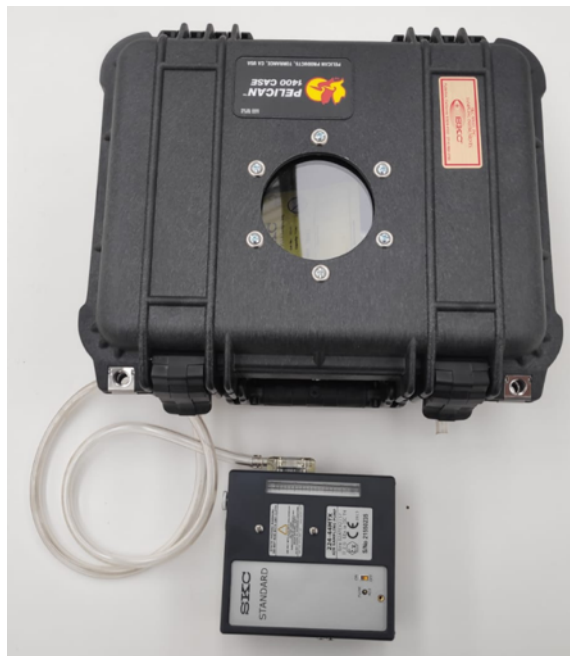
Annex X. 5 Vac-U-sampler used with a SKC standard air pump
