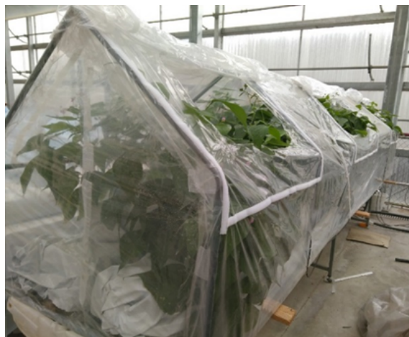
Figure 2. 5 Closed chamber during N 2 O emission experiment with green beans
