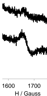
Figure 3-12. EPR spectra of |\Delta m_s| = 2 transition at half-field for the same concentration 10^{-4} M of G0-OEG-
