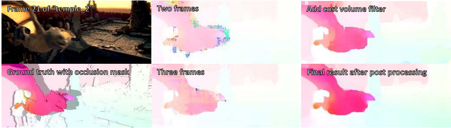
Figure 5.5 – Discrete optical flow results on the MPI-Sintel training dataset for two frames, three frames and three frames with cost volume filtering; final flow values after post-processing.
