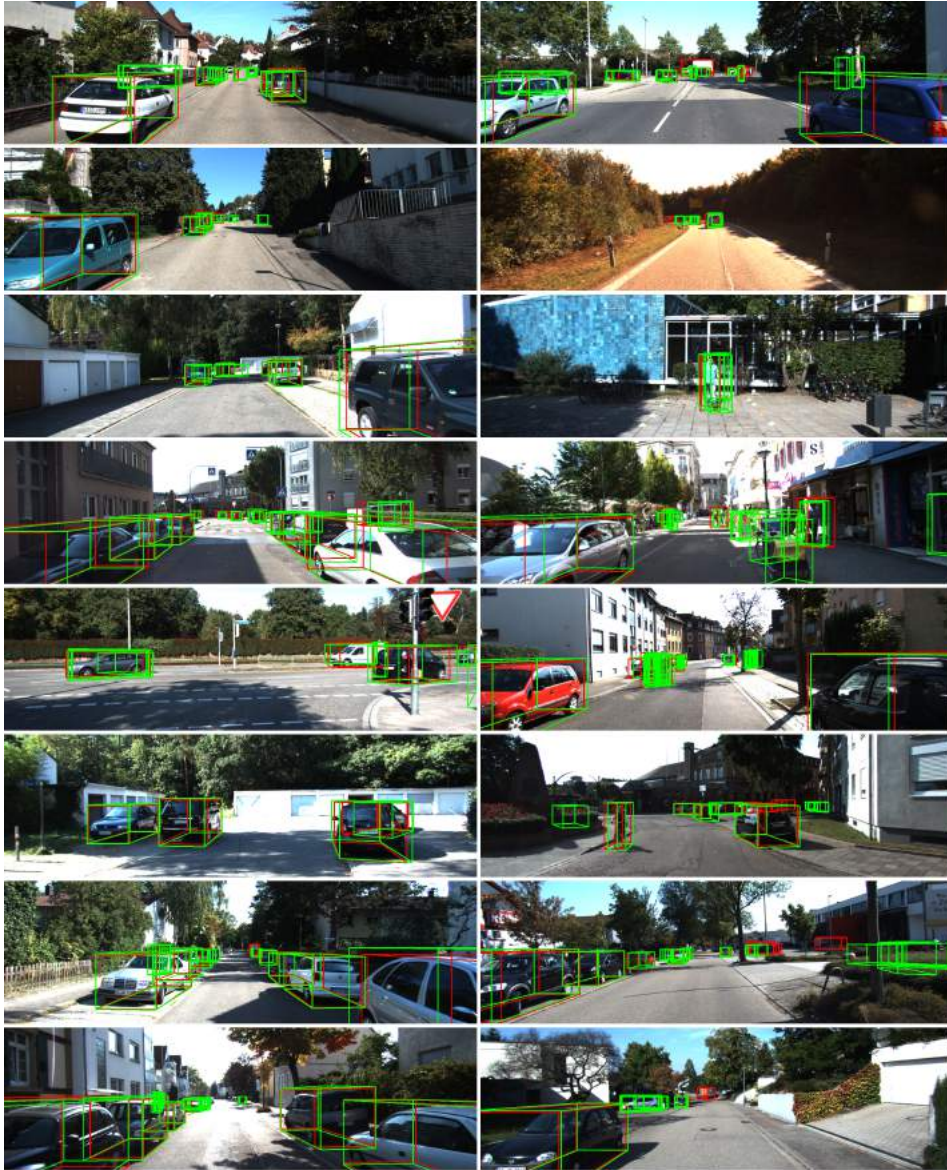
Figure 4.13 – 3D object detection based on MonoDELSNet-St combined with CenterPoint. Red BBs are ground truth, green ones are detections. Detections are shown for cars, pedestrians, and cyclists.
