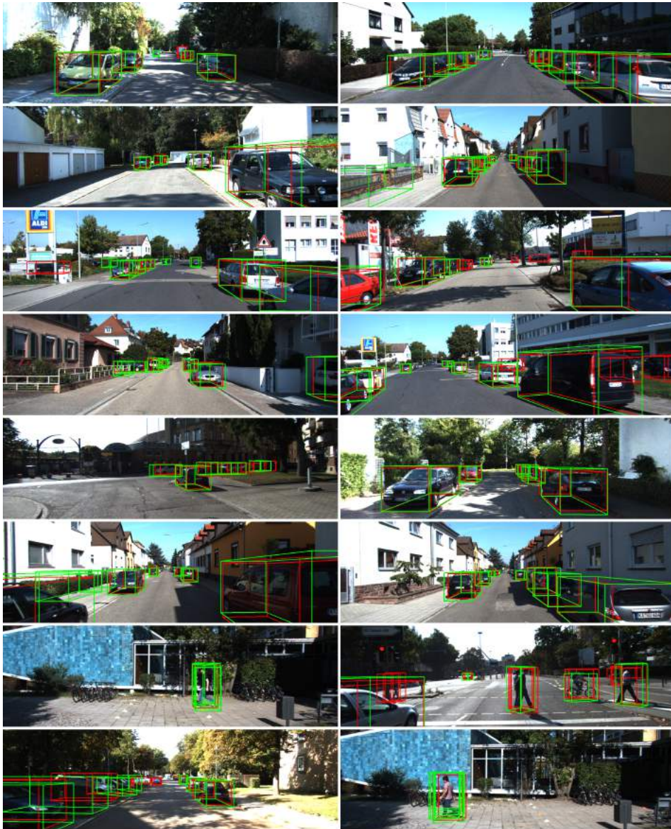
Figure 4.11 – 3D object detection based on MonoDELSNet-St combined with Point R-CNN. Red BBs are ground truth, green ones are detections. Detections are shown for cars, pedestrians, and cyclists.
