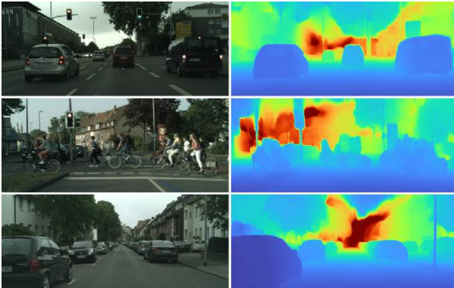
Figure 3.10 – Qualitative results of MonoDEVSNet on Cityscapes dataset. From left to right: input images, MonoDEVSNet estimated depth maps.
