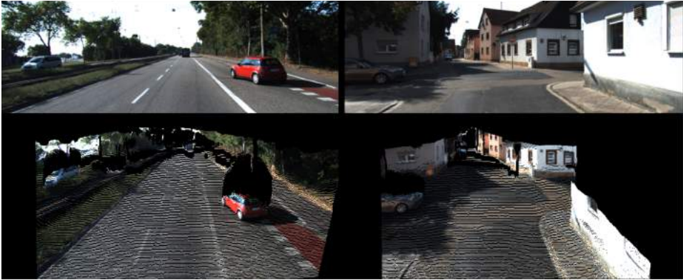
Figure 3.7 – Point cloud representation on KR Eigen test split [30] and KS data from left to right. From top to bottom: input images, MonoDEVSNet textured point cloud.
