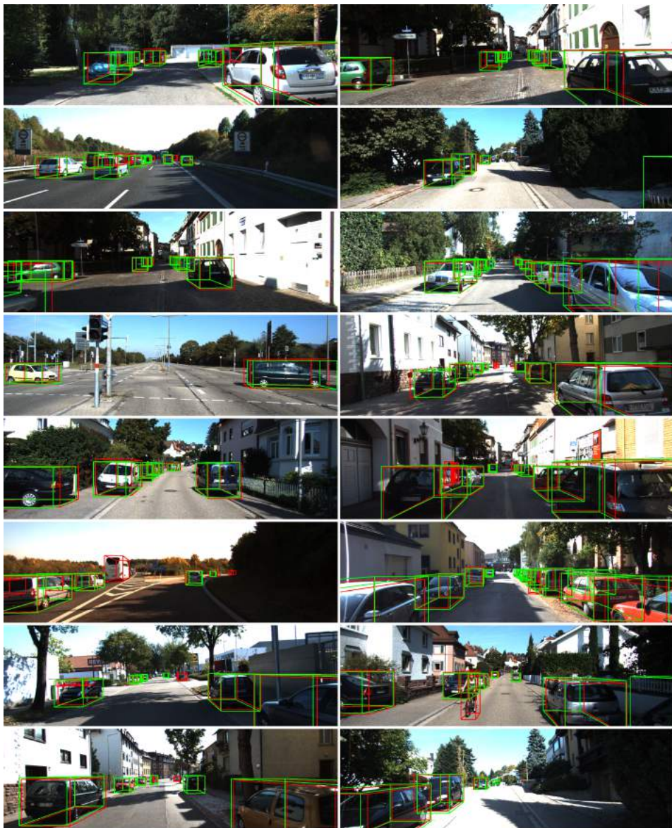
Figure 4.12 – 3D object detection based on MonoDELSNet-St combined with Voxel R-CNN. Red BBs are ground truth, green ones are detections. Detections are shown for cars.
