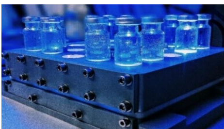
Figure 3. 45. In-house developed parallel photoreactors with 25 positions for vials of 10 or 21 mL.
