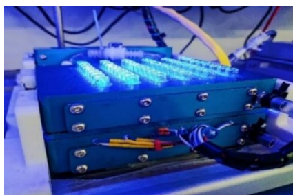
Figure 3. 46. In-house developed parallel photoreactors with 48 positions for vials of 1 mL.
