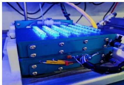
Figure 5. 7. In-house developed parallel photoreactors with 48 positions for vials of 1 mL.
