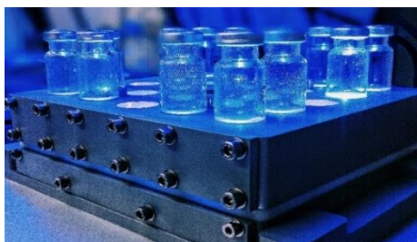
Figure 4. 15. In-house developed parallel photoreactors with 25 positions for vials of 10 or 21 mL.
