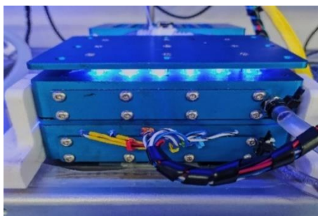
Figure 4. 16. In-house developed parallel photoreactors with 48 positions for vials of 1 mL.
