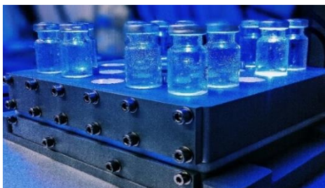
Figure 5. 8. In-house developed parallel photoreactors with 25 positions for vials of 10 or 21 mL.
