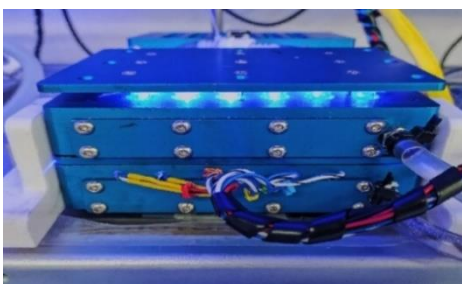
Figure 3. 46. In-house developed parallel photoreactors with 48 positions for vials of 1 mL.
