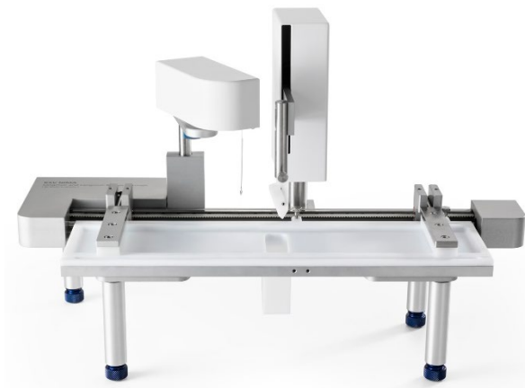
Figure 7. A Langmuir-Blodgett trough with an extractor. Any part that could be in contact with the buffer or the lipid monolayer: the reservoir, the barriers and the tweezers made of Teflon®.
