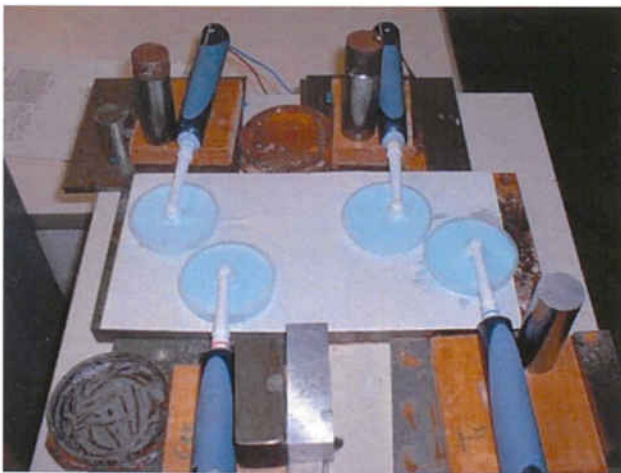
Fig. 1 The materials tested immersed in toothpaste slurry and placed into four plastic recipients are submitted to brushing by four units of electric toothbrush which are fixed to platforms subjected to a 250 g load
