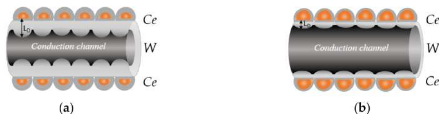
Figure 11. The schematic view of the heterojunction formed at the surface of the cerium oxide ( Ce ) core-shell tungsten oxide ( W ) wires and the possible mechanism (a) after exposure to air and (b) reducing gases such as acetone. L_D is the Debye length or depth of the depletion region from the surface (not at scale).
