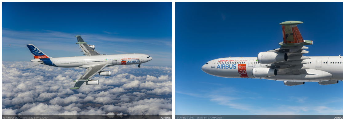
Figure 1.1. BLADE project A340 flight test with laminar aerofoils in the outer wing sections (Ramadier, 2017).
