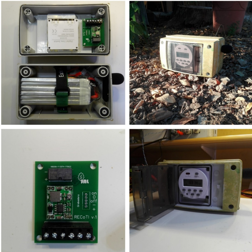
Figure 1. Photos of the RECoti ARU where it can be seen its interior with the Lipo battery, the motherboard, and the programmer, all protected within the waterproof case.
