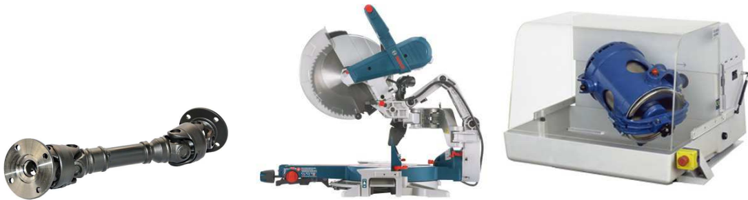
Figure 4.5: Industrial applications of overconstrained 6R mechanisms. From left to right: A double-Hooke's-joint transmission, a Sarrus linkage used in the positioning of a Bosch saw, and a Turbula mixing machine based on the overconstrained mechanism proposed in [155].
