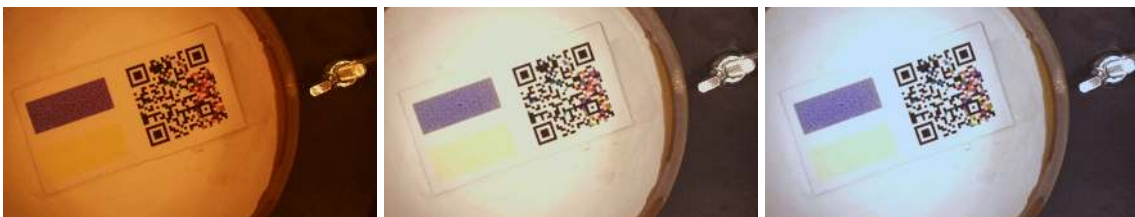
Figure 6.19: A printed sensor, featuring a Color QR Code and two colorimetric indicators is displayed inside the sensor chamber of our setup. Then is exposed to different light conditions. From left to right, the illumination changes following 3 color temperatures of white light: 2500K, 4500K and 6500K.
