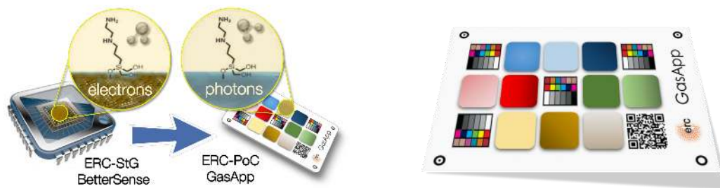
Figure 1.1: The GasApp proposal is presented. Left, GasApp changed the core sensing technology from electronic to colorimetric indicators. Right, the initial idea of the GasApp project, a card where colorimetric dyes are printed alongside with color charts and a QR Code.
