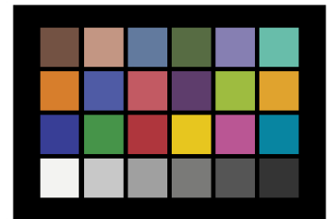
Figure 2.3: A ColorChecker chart. The first row shows a set of six “natural colors”; the second one shows a set of “miscellaneous colors”; the third, primary and secondary colors; and the last row, a gray scale gradient. This set of colors samples the RGB space in a limited way, but it is convenient to carry out a few color corrections manually.
