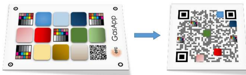
Figure 1.4: Our thesis proposal to create machine-readable patterns that can accommodate colorimetric sensors and color charts, alongside with the digital information of the QR Code.
