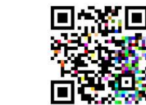
Figure 6.11: A back-compatible Color QR Code for colorimetric indicators. This QR Code will be read by commercial scanners, and it should display the URL: c-s.is/#38RmtGVV6RQ5f . The Color QR Code includes up to 125 reference colors and blank space to allocate a colorimetric indicator ink (above the lower finder pattern).
