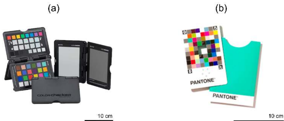
Figure 2.4: Previous state-of-the-art color correction charts from Pantone and X-Rite. (a) The X-Rite ColorChecker Passport Photo 2 ® kit. (b) The Pantone Color Match Card ® .
