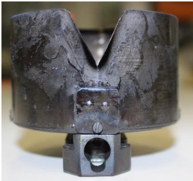
Figure 3.20. a) Front view of the sample holder showing the locking position and b) the arm that we use to lock the sample holder.
