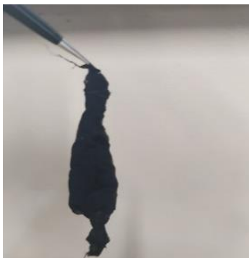
Figure 6.8. CNTs mat obtained by FC-CVD process
