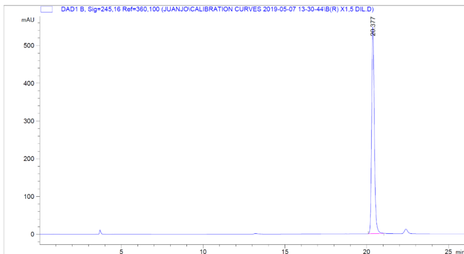
Figure 125. HPLC chromatogram of enantiopure ( R )- B1 . Conditions: CHIRALPAK® IC, n -Hex/IPA 99:1 to 95:5, 1 mL min -1 , gradient (min, %IPA): (0, 1); (7, 1); (14, 5); (40, 5).
