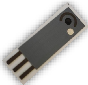
Figure 5.16. A new electrode design with a smaller working electrode and a round reference electrode.
