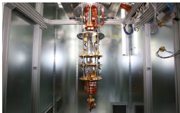
Figure 8.13: Inside D-Wave Quantum Computer [104]
