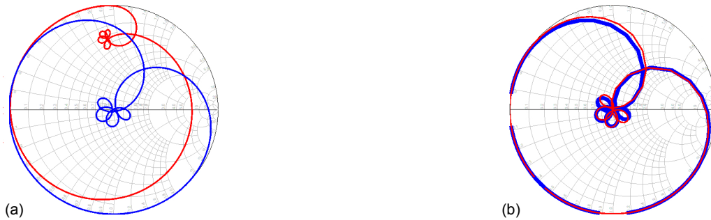
Figure 5.2: Reflection coefficient representation of filters with Z_{in} = 50 \Omega (blue) and Z_{in} \neq 50 \Omega when (a) Z_S = 50 \Omega and (b) Z_S = Z_{in}^* \Omega .
