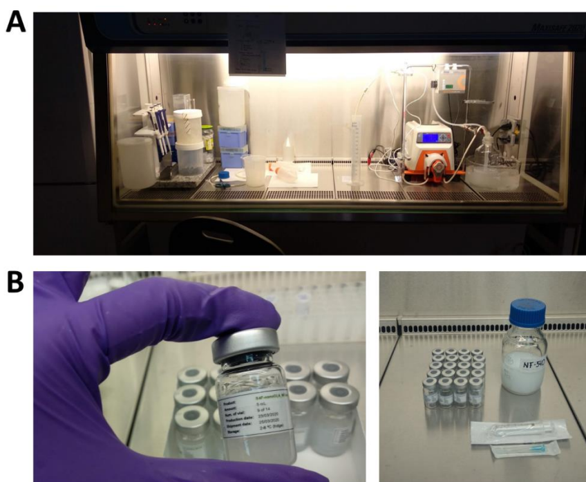
Figure 6.27. (A) Setting of the TFF process in a laminar flow cabinet to maintain a sterile environment, and (B) aliquoting of nanoGLA in sterile vials (see Chapter 9.16.3 ).
