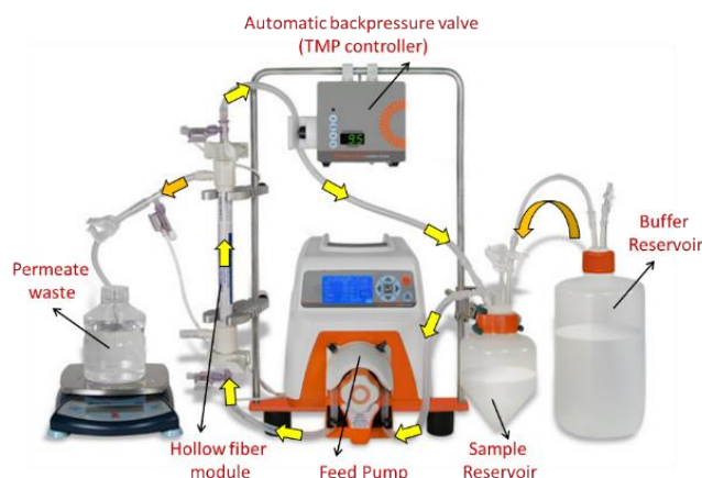
Figure 9.4. Schematic set up of KrosFlo Research Iii TFF System , used for diafiltration purification step. Adapted from manufacturer’s operating instructions. 1
