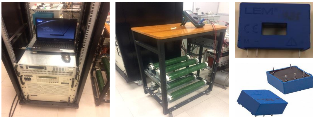
Fig. F.5 Experimental components smart source, resistive load, current and voltage sensors
