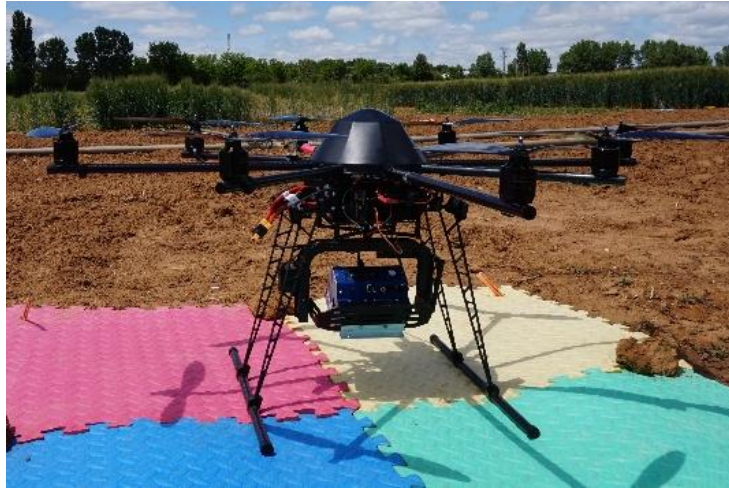
Figure 4. OktoXL 6S12 unmanned aerial platform equipped with the Tetracam multispectral sensor.
