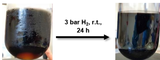
Figure 3. Picture of the starting reaction medium before hydrogenation (left) and crude colloidal suspension of bimetallic RuCo NPs obtained after hydrogenation (right).
