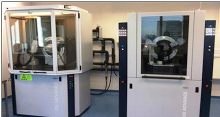
Figure 3.15. XRD Bruker D8 A25 Advance used for XRD quantitative analyses.
