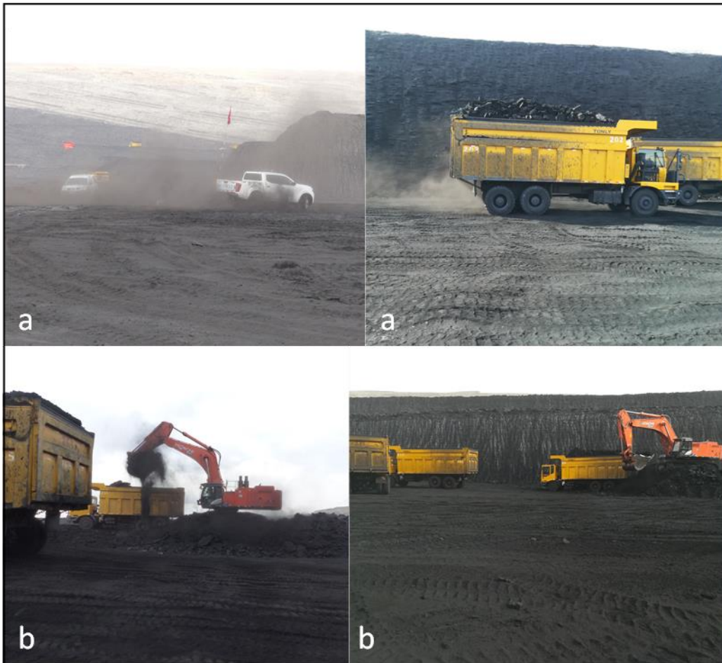
Figure 3.6. a) Resuspension of coal dust at CWFs, due to the transportation of coal; b) dust emitted due to handle coal, uploading coal after drilling the coal face.
