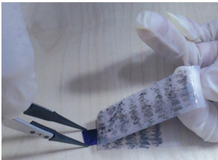
Figure 2: Scotch tape method of graphene synthesis from graphite. Reproduced from [10] with permission from Springer Nature.
