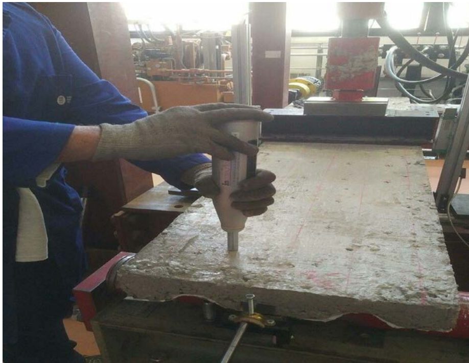
Figure A. 9. Implementing of rebound hammer test for compressive strength.
