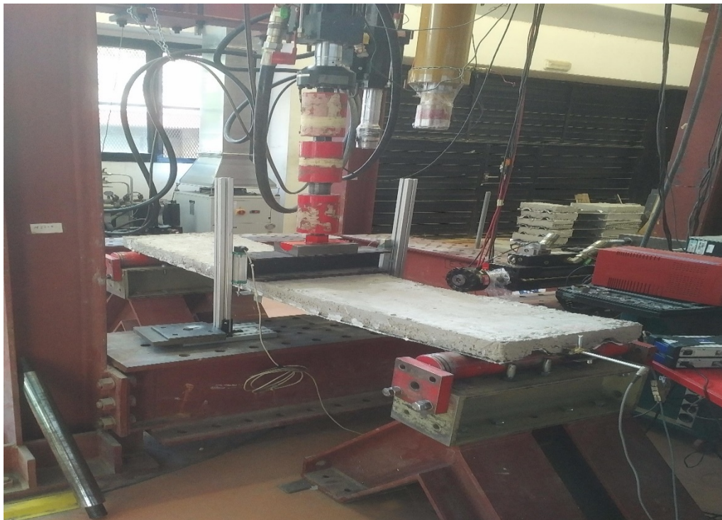
Figure A. 3. Three-point bending test method.
