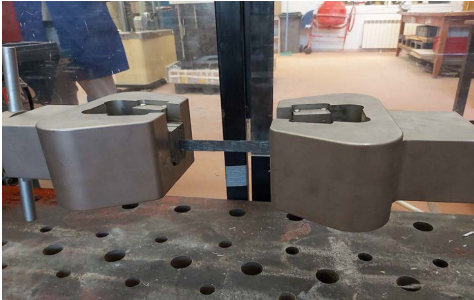
Figure A. 10. Implementing of ASTM D638 test for tensile strength.
