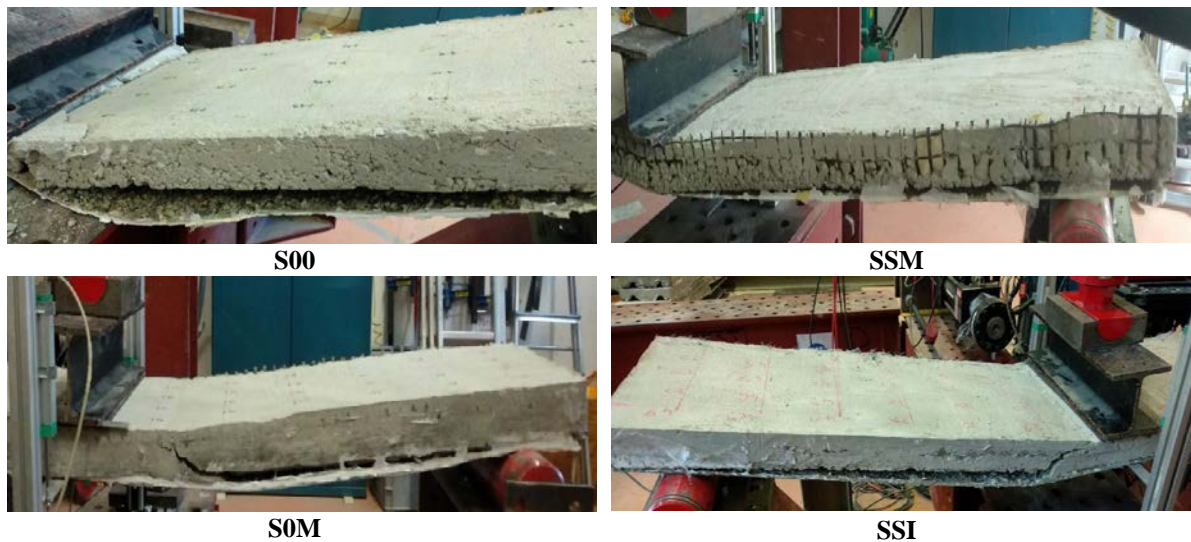
Figure 22. Typical failure mode of all specimen types
