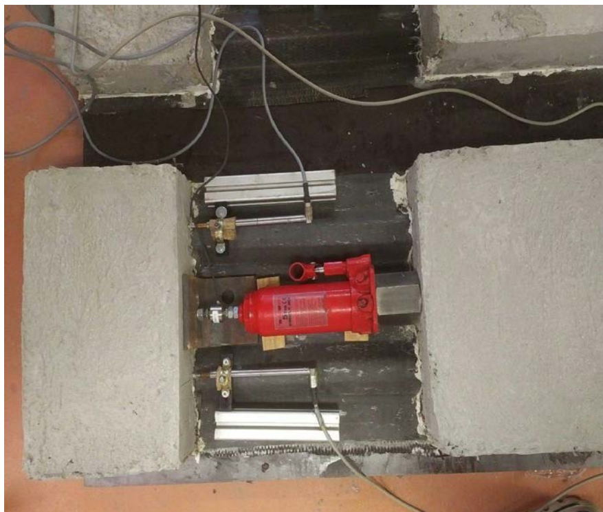
Figure A. 6. Shear setup configuration.
