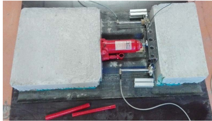
Figure 26. Shear test setup configuration
