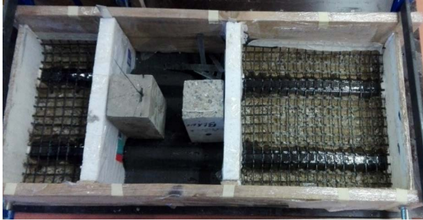
Figure 23. Formwork and CFRP connection of specimen S0M-1 before pouring concrete
