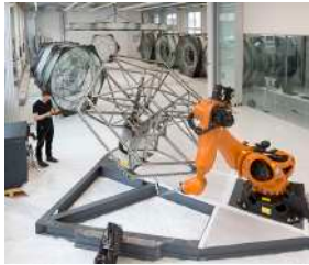
VI.9_Glass-and-carbon-fibre-cell-Elytra-Filament for the V&A museum Pavilion, London, Archim Menges_2016
