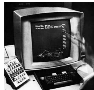
2.5.1-3_A13-URBAN 5 system, the user making selections with the light pen in dialogue with the system,1968
