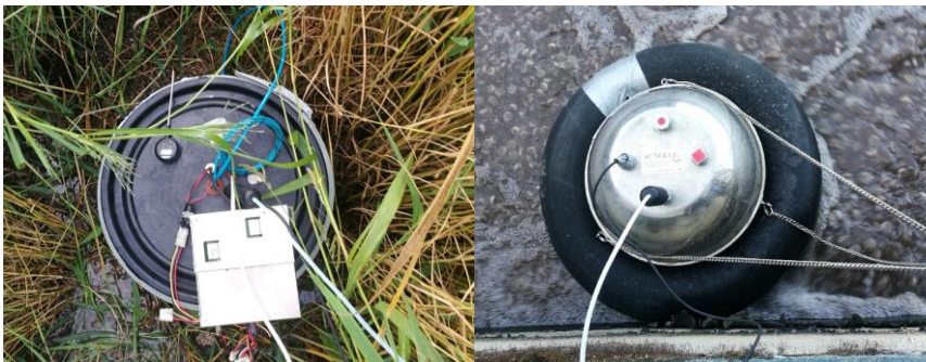
Figure A. 4. Greenhouse gas measurements using the static chamber method in constructed wetlands (left) and the floating chamber method in the activated sludge system (right)
