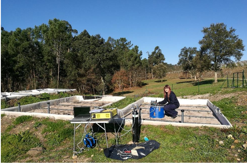
Figure A. 1. Set up for the measurement of greenhouse gas emissions in the vertical subsurface flow constructed wetland with the FTIR gas analyser.
