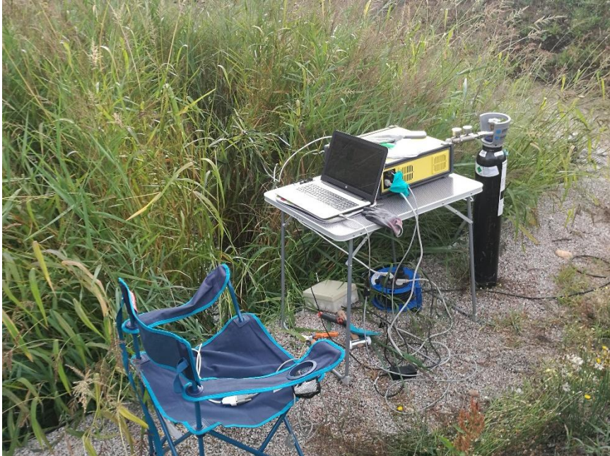
Figure A. 3. Set up for the measurement of greenhouse gas emissions in the horizontal subsurface flow constructed wetland with the FTIR gas analyser.
