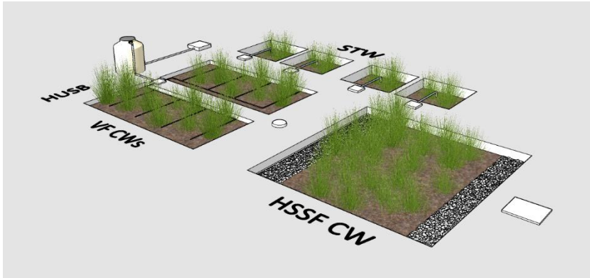
Figure 6.1. 3D representation of the constructed wetlands (CWs) system in the winery located in Galicia (Spain). HUSB – hydrolytic upflow sludge blanket reactor, VF – vertical flow CWs, HSSF – horizontal subsurface flow CW, STW – sludge treatment wetlands.
