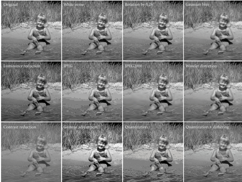
Figure 7.1. Original and 11 distorted images, from the CSIQ database. All distorted images have a PSNR of 22.5 dB, however, there exists a large variation in perceived quality between images.
