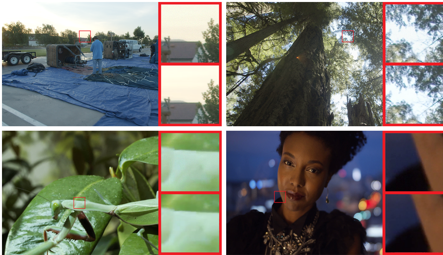
Figure 6.7. Screenshots of the four sequences used in the subjective assessment, with optimal amount (in terms of image appearance) of retinal grain added. Each image shows a zoomed-in region (marked with a red square) in two versions, with (top) and without (bottom) the retinal grain. From left to right, top to bottom: "Balloon", "Nature", "Bugs", and "Closeup".
