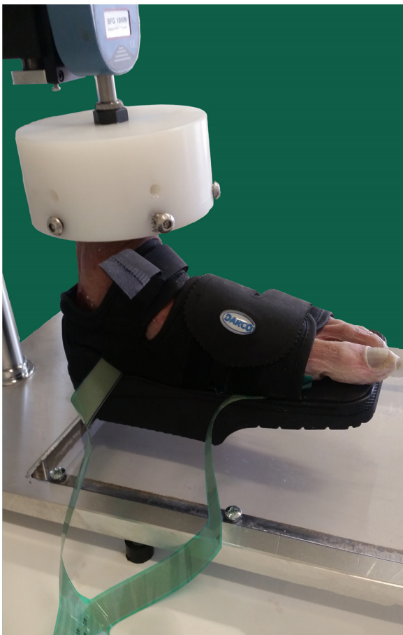
Fig. 4. Specimen with the postoperative shoe attached to torque-based force bench. It is possible to observe the placement of the sensors for data collection between the sole of the foot and the shoe.
