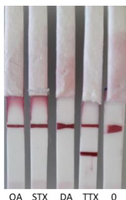
**Figure 4.5.** Cross-reactivity experiment for the dipstick experiment using 4 different marine toxins (OA, STX, DA, and TTX).
