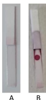
**Figure 3.2.** Optimization of control line DNA probe. In this experiment 0.4  $\mu\text{L}$  (100  $\mu\text{M}$ ) of each aminated probe was directly immobilized on control line via UV-crosslinking (A) Using aminated docking probe. and (B) Using aminated reverse prime.
