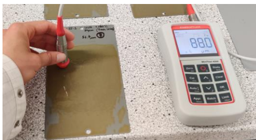
Figure 4.8. Thickness measurement of a dry coating.
