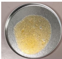
Figure 4.14. Aluminum tray with a film after thermal curing corresponding to a 1:1 alkene:thiol ratio.
