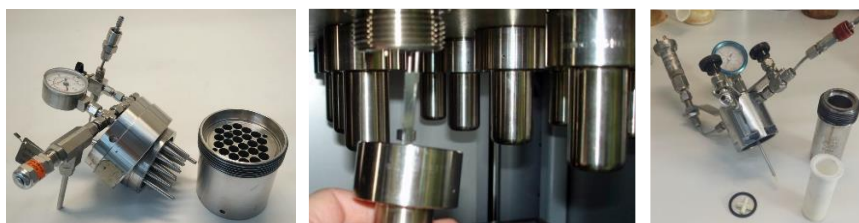
Figure 2.5. High pressure reactor systems used to achieve the results of this chapter: a HEL (left), AMTEC (middle), and standard autoclave high pressure reactor system (right).
