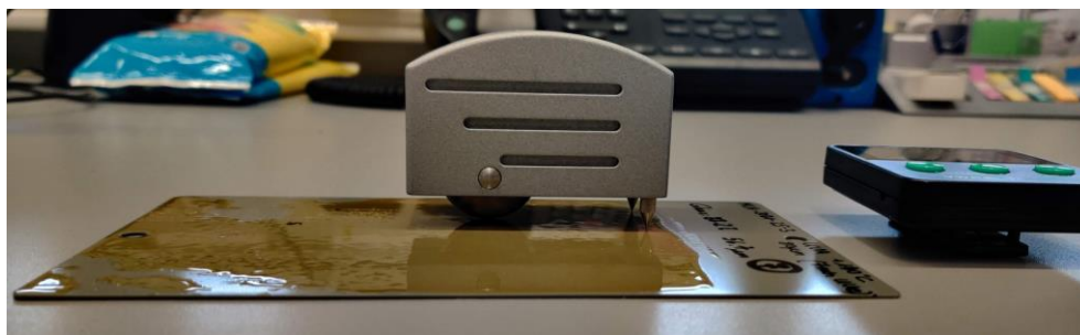
Figure 4.10. Buchholz hardness indenter placed on the surface of a panel to perform a hardness test.
