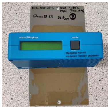
Figure 4.7. Reflectometer measuring the gloss of a coating sample.
