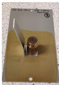
Figure 4.6. Dryness test example with an “L” shape metal piece placed in the middle of the panel containing the coating.
