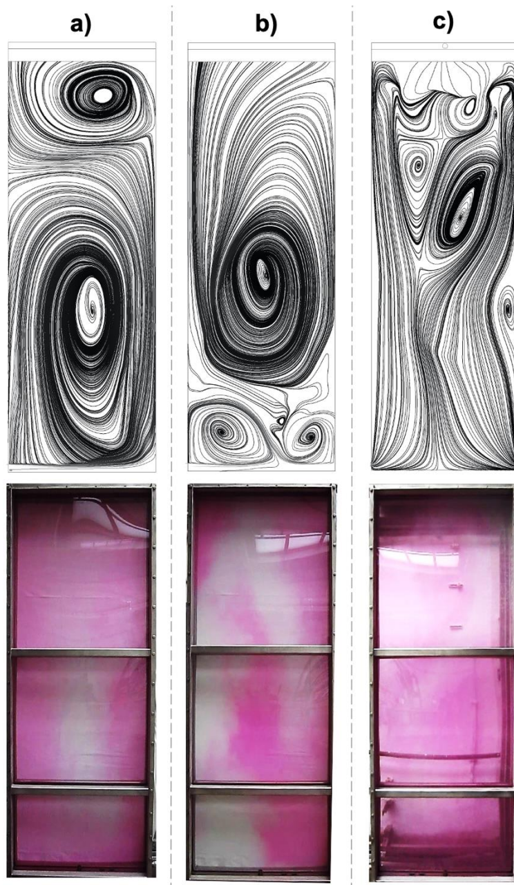
Fig. 7.2.2.2. Calibration of CFD model. Comparison of tracer experimental measurement method (on the bottom) and numerical simulation of streamlines (on the top) – flow rate: 45 \text{ L min}^{-1} . a) single bottom inlet and top outlet, b) double bottom inlet and top outlet, c) top inlet and double bottom outlet.
