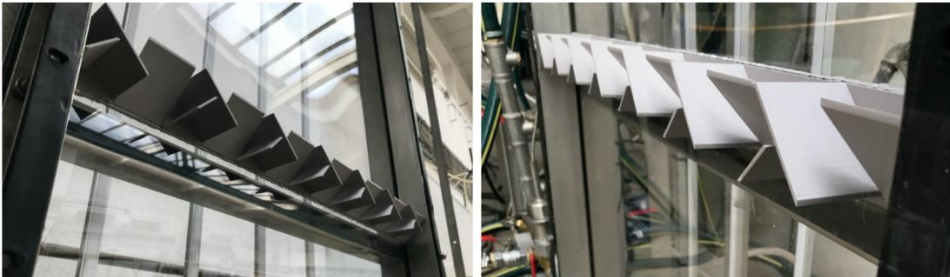
Fig. 8.1.3. Static mixer in FP PBR chamber.
