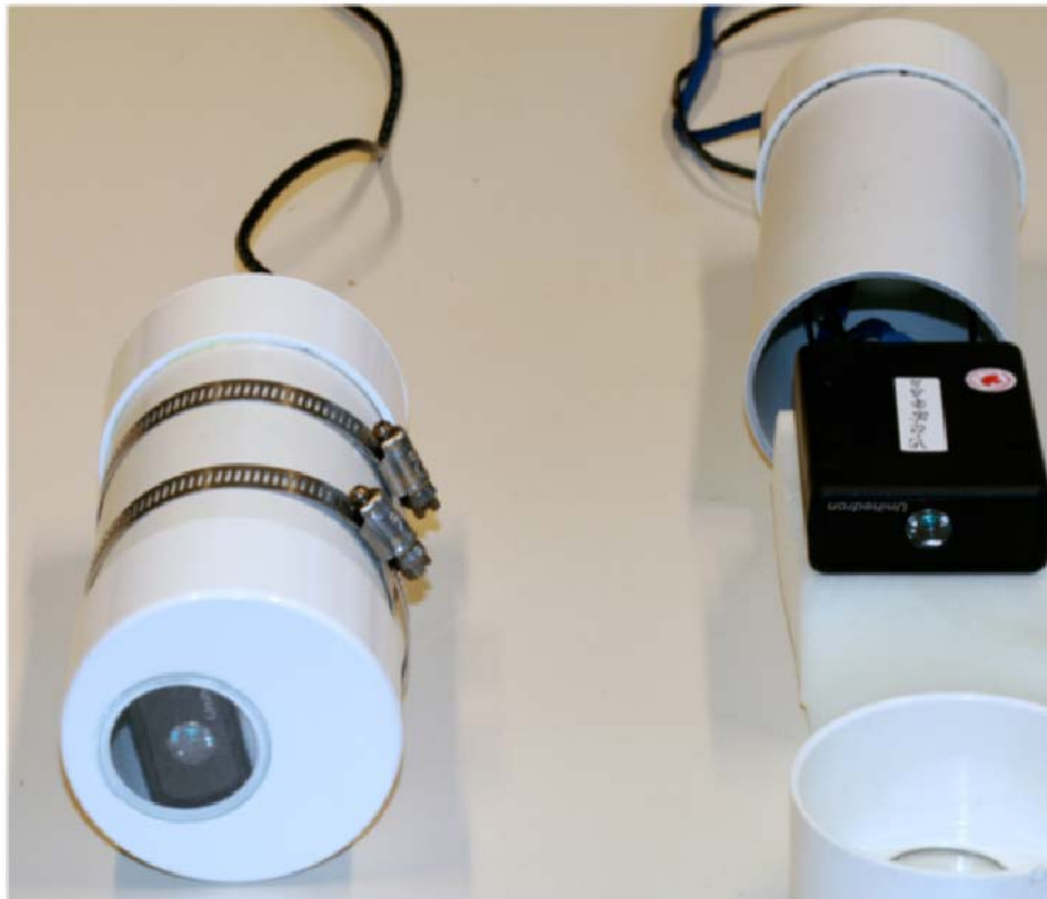
Figure 2.3: Two SQM. Right: inside its housing. Left: partially outside its housing. Image from Kyba et al. (2011).
